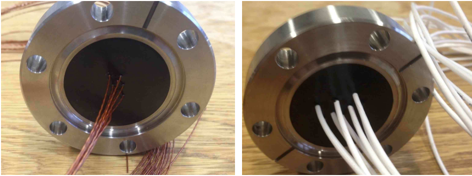
FIG. 4.10 – Example vacuum feed-throughs for 10 high voltage and 10 signal cables.
