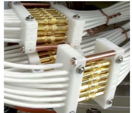
FIG. 4.9 – Custom-made connectors for XENON1T. Above: High voltage connector with Kapton cables and strain relief. Right: Signal coaxial cables with MMCX connectors in a PTFE holder structure.
