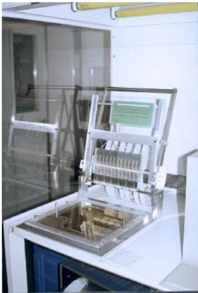
Figure 4.4: Photograph of the electrical MSGC anode break tester, designed by and built at the University of Zürich, during testing of the first larger series of HERA-B substrates at IMT (Greifensee). The cover, which contains the electronics board and anode contacts, is open. When it is closed and locked, contact is being made. The whole installation is within a clean box.
