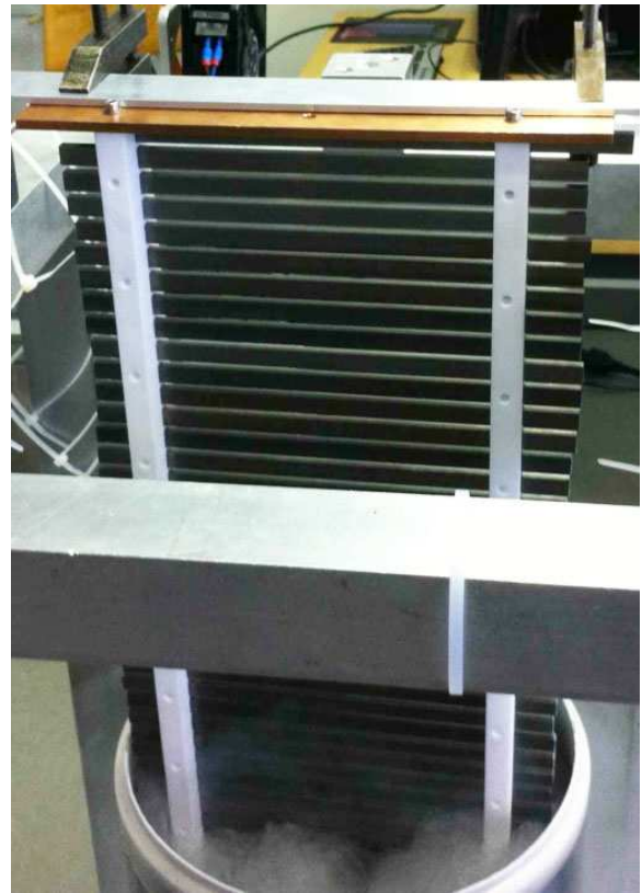
FIG. 4.3 – The 1:16 scale mockup using stainless steel field shaping rings during a cryogenic test in LN.
