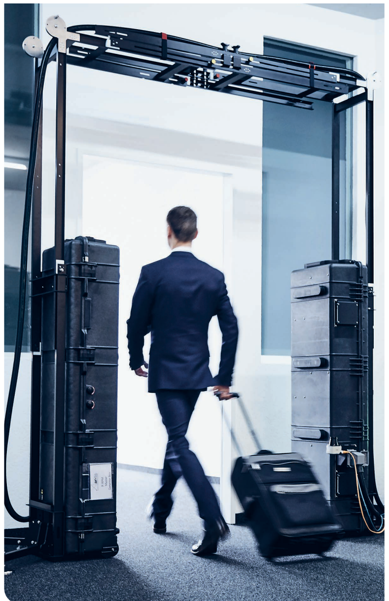
Figure 24: A Radiation Portal Monitor that screens passing pedestrians and their luggage for illicit radioactive sources, developed by Arktis Radiation Detectors Ltd, a spin-off from particle physics research at ETH Zürich. Swiss authorities use systems like this for spot checks at airports ( www.arktis-detectors.com ) (Image: R. Chandra/Arktis)
