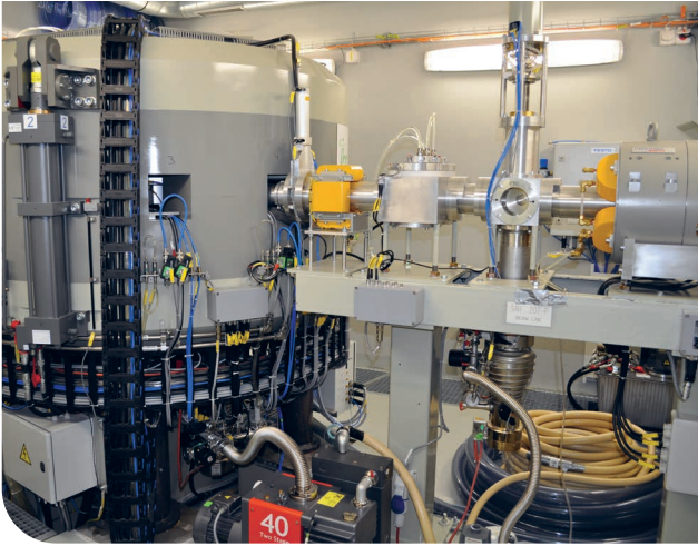
Figure 25: The medical cyclotron by SWAN Isotopen AG in operation at the Uni Bern hospital, Inselspital, with its unique beam transfer line for research, including medical applications of particle physics techniques (Image: S. Braccini/Uni Bern)
